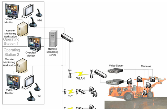
Figure 1. Overall architecture of Sandvik's remote monitoring system of a drill machine.
